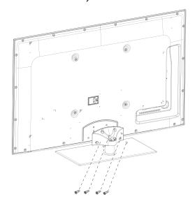
3 Secure the stand to your TV using the provided four screws.
